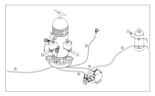
During installation the pump pressure must be set at 9 bar. This pressure is shown on the pressure gauge when the machine is dispensing.
