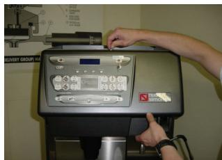
Insert key and unlock door of the machine.
