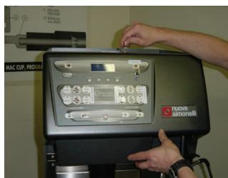
Once chamber has been cleaned close door and lock it. Take key out of lock.
