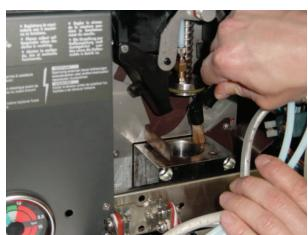
Clean chamber surface and piston with brush that has been provided.
