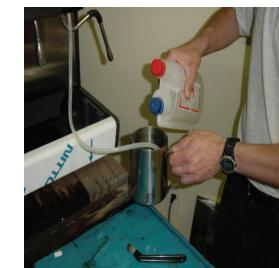
Machine will wash for 5 mins during this cycle the puly milk will empty please refill with fresh clean water.
