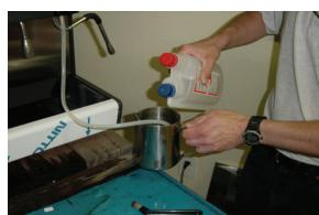
Mix Puly milk solution for cleaning milk foamer according to directions on bottle.
