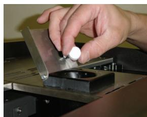
Open decaffe chute and put Puly tablet in to chute. Close decaffe chute.
