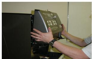
Lift door straight up to lock position to gain access to brewing chamber.
